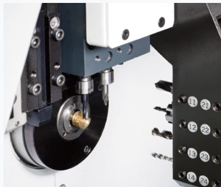
▶ Main & Sub-spindle simultaneous drilling and tapping
