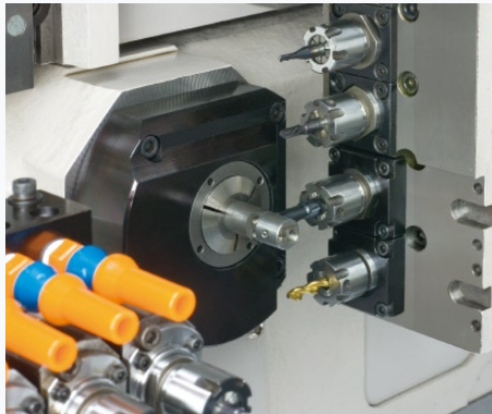
▶ Main & Sub-spindle simultaneous drilling and tapping
