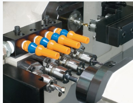
▶ Rear offset drilling and tapping
